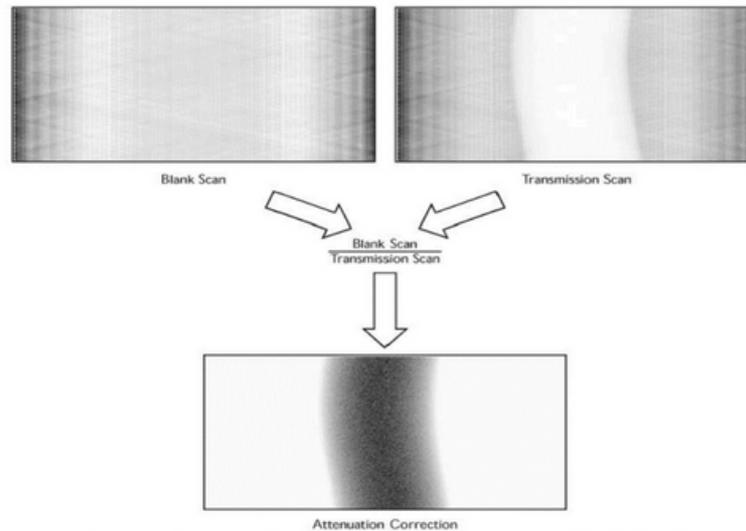
**Figure 2** : Showing the attenuation correction matrix which is obtained by dividing the blank scan sinogram (acquired without the subject in the scanner) by the transmission scan sinogram (acquired with the subject in scanner) [8].
