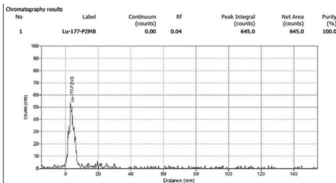
**Figure 1** : The radiochemical purity of the radioconjugate [Lu-177]Lu-DOTA-pertuzumab estimated by thin layer chromatography.
